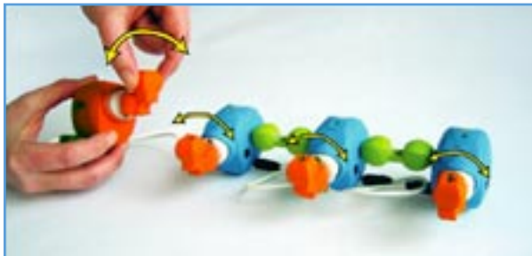
Programming with a Queen: In both record and playback modes, all motions of the Queen are imparted directly to all Actives connected to the Queen.
